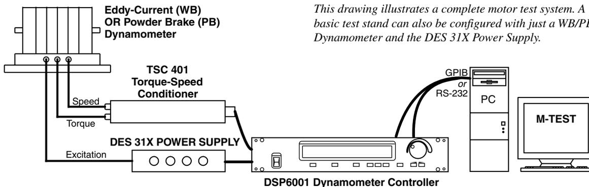
*This drawing illustrates a complete motor test system. A basic test stand can also be configured with just a WB/PB Dynamometer and the DES 31X Power Supply.*
