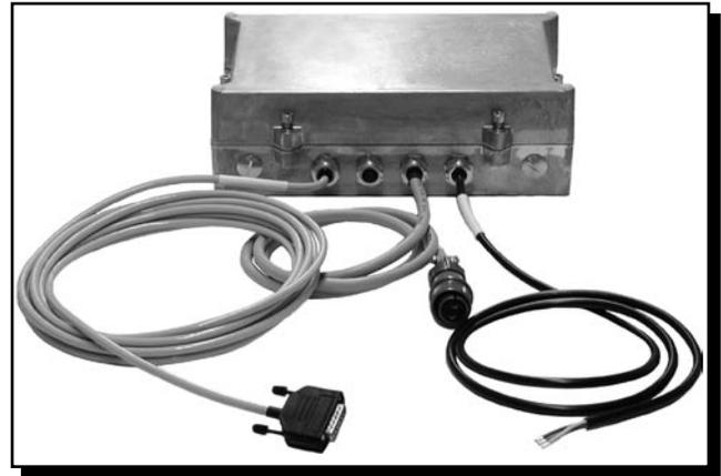
There are two digital outputs (alarms): one is an electrical fault indicator and the other detects overheating in the DES unit or the cooling water. If one of the alarms is activated, a general alarm is signalled by means of relay contacts.
