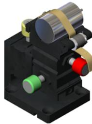
Attached to the dynamometer base plate is a motor fixture designed expressly for micro/miniature motors. The base of the fixture features an XYZ stage with 3-axis positioning for excellent adjustability and motor centering. With the included adapters, motors from 5 mm to 30 mm in diameter can be easily mounted. The fixture is keyed to help secure the motor under test and a rubber strap with knurled cam grip provides motor clamping.
