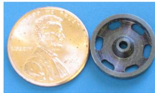
Figure 5–2 Micro Dyne Rotor
