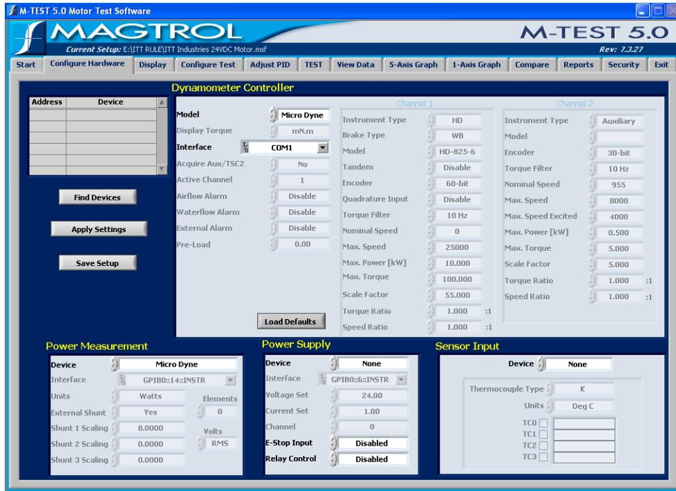
Figure 4–4 M-TEST Configure Hardware Window
