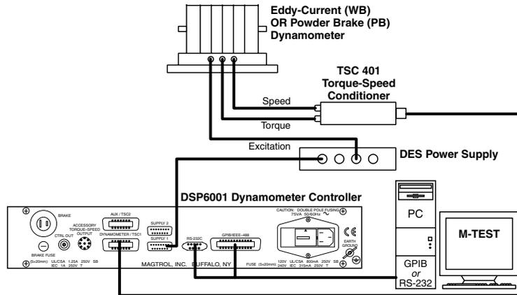
Magtrol also offers In-Line Torque Transducers, which employ a unique non-contact differential transformer torque measuring technology providing extremely accurate torque and speed measurement with superior electrical noise immunity. For a dynamic, high-precision system, the torque transducer can be mounted in line between the unit under test and the dynamometer.
