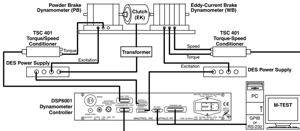
**EDDY-CURRENT DYNAMOMETER OPERATING PRINCIPLES**
