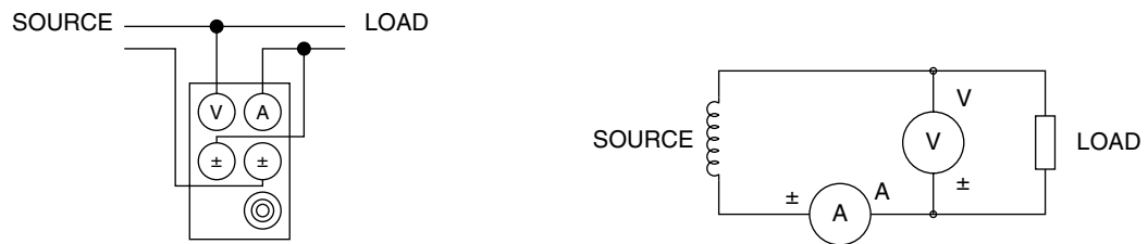
Figure 3-7 Single-Phase, Two-Wire Wiring Schematic
